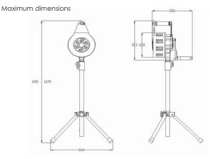
Stand height: max 1m, min 0.6m When folded: height 0.2m, base tripod 0.03m x 0.03m x 0.03m
