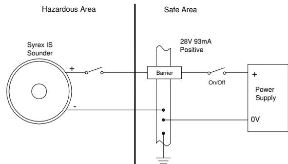
Fig 4 Single stage alarm using single channel barrier.
